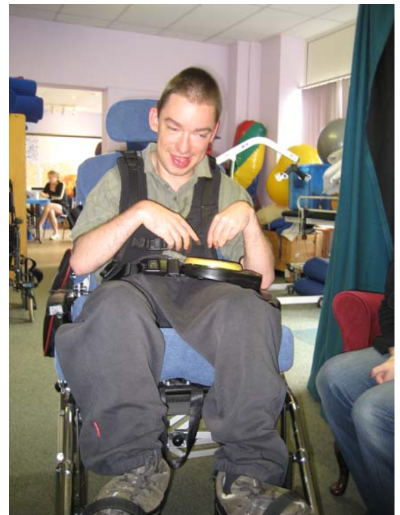
Many of the people who use Parity's services do not use speech to communicate. Equipment like the 'big mack' switch above carry a recorded message which plays when the device is pressed, so the person can make a choice such as 'yes' or 'no'.
